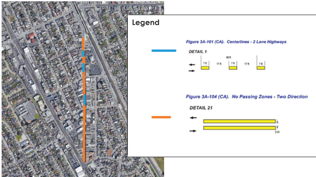
Figure 1: Centerline Marking Recommendations
