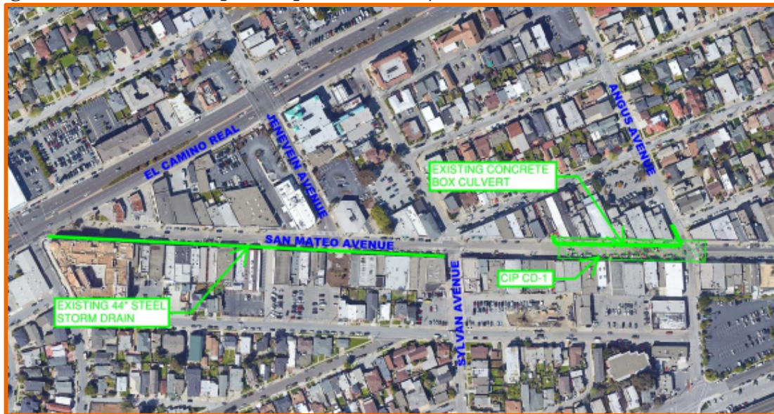
Figure 3: Storm Drain Capital Improvement Project Location
