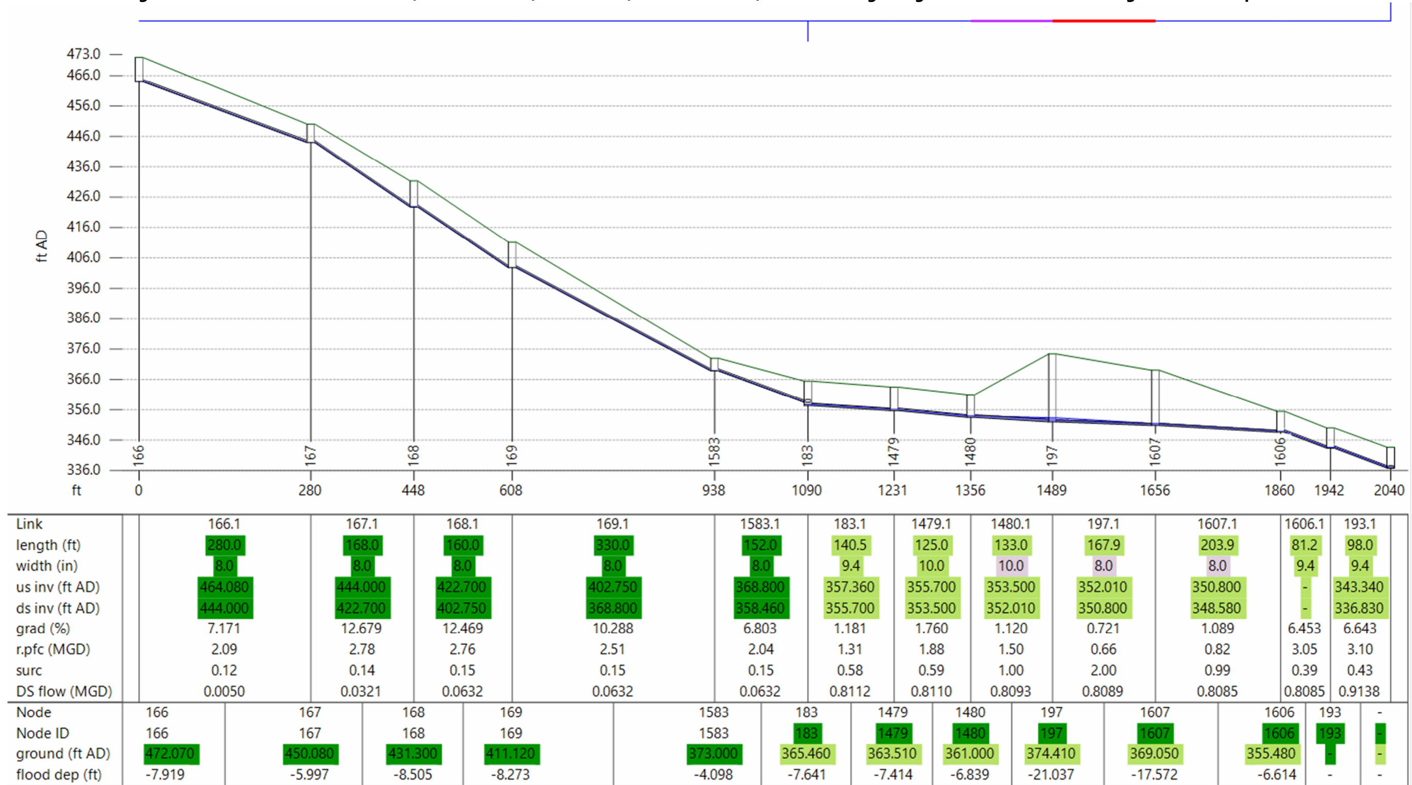
Figure 2: Model Profile from MH166 (Glenview Drive) to MH191 (Claremont Drive) under Existing Design PWWF with Glenview Highlands Development
